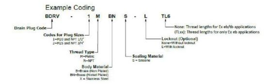
Note: (Thread Length) in the key code is mandatory for products having thread length different than the minimum TL for ex eb/tb applications indicated in the assembly tables.
