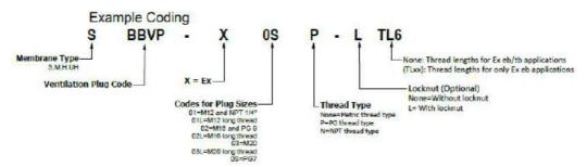
Note: (Thread Length) in the key code is mandatory for products having thread length different than the minimum TL for ex eb/tb applications indicated in the assembly tables.
