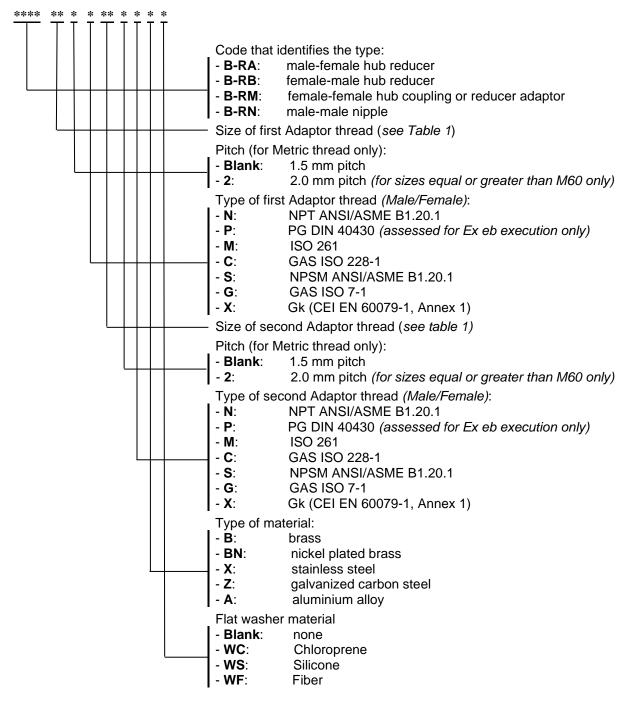
The Adaptors type **B-RM** and **B-RN** have both NPT threads or both Metric threads or coupling NPT-Metric threads.
