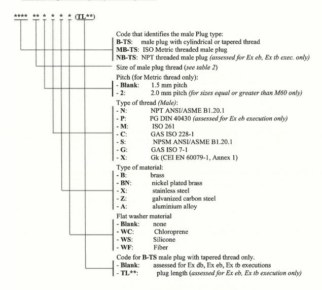
The sizes and thread types of the Adaptors and Plugs are listed on the tables below:
