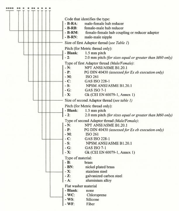
Adaptors type **B-RM** and **B-RN** have both NPT threads or both Metric threads or NPT-Metric coupling. Adaptors type **B-RB..**, **B-RM.** and **B-RN.** can be made with the combination of two different types and sizes of threads or with the same combination.
